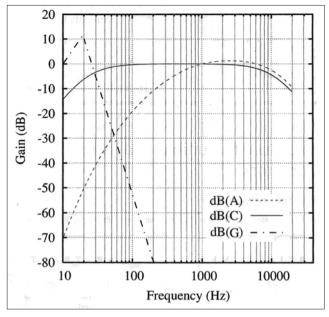
Figure 1. Frequency characteristics of G and LIN filters applied in infrasonic noise measurement applied in working environments [11, 12, 13, 14, 15]
